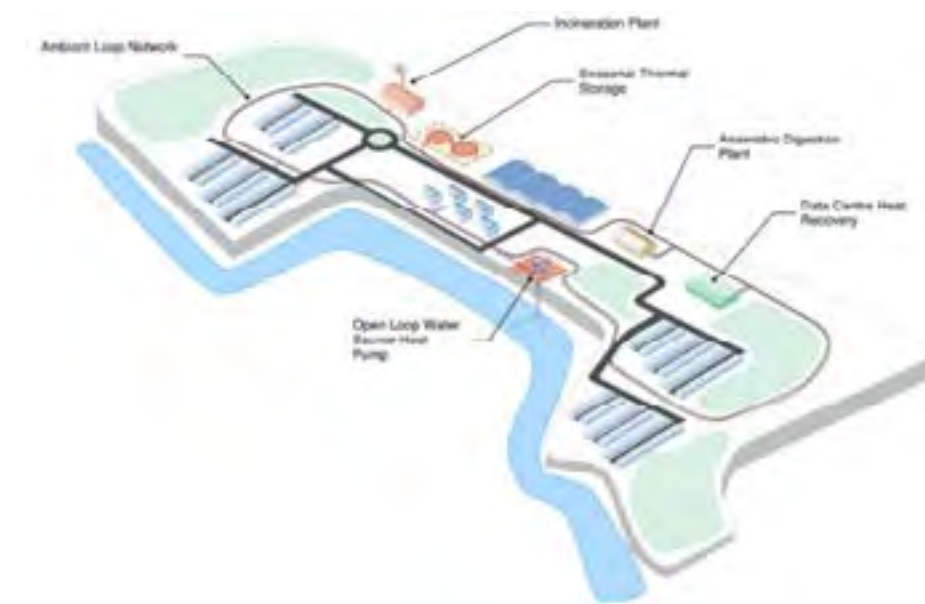
Fig 42 5G Ambient Loop District Heat Network
