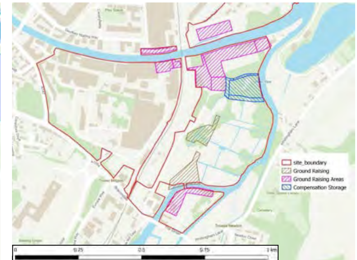
Fig 46 Ground raising compensatory storage areas to enable masterplan delivery
