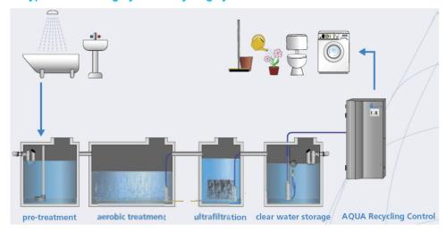
Combined rainwater harvesting and greywater recycling systems can be particularly effective, with the use of rainwater supplementing greywater flows at peak demand times (e.g. morning and evenings).
