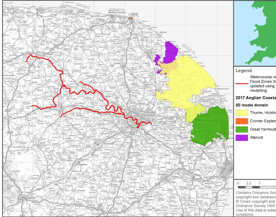
Figure 1-2: Coverage of hydraulic models where the outputs were used to update Flood Zones 2 and 3a
